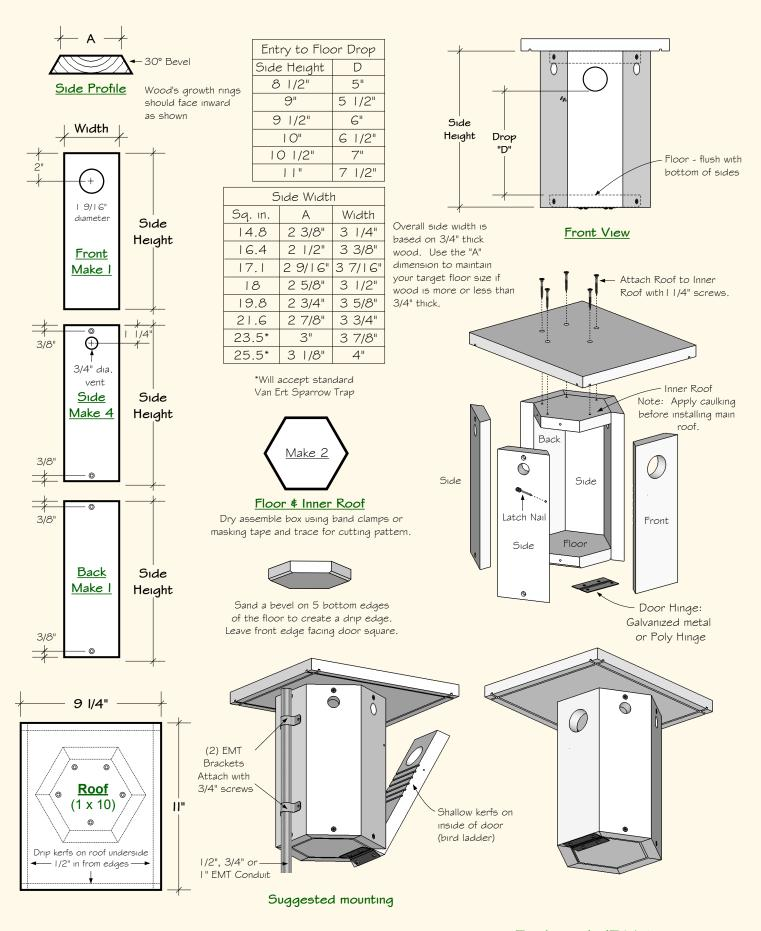
Material: Sides for boxes with floors up to 17.1 sq. in. can be cut from 1 x 4 (3/4" x 3 1/2"). Boxes with floors 18 sq. in. and over require a 1 x 6 (3/4" x 5 1/2"). Floors and Inner Roof for all sizes require 1 x 6. Roof is 1 x 10 (3/4" x 9 1/4").
